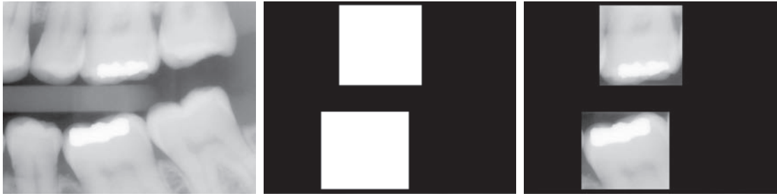
FIGURE 2.34 (a) Digital dental X-ray image. (b) ROI mask for isolating teeth with fillings (white corresponds to 1 and black corresponds to 0). (c) Product of (a) and (b).
