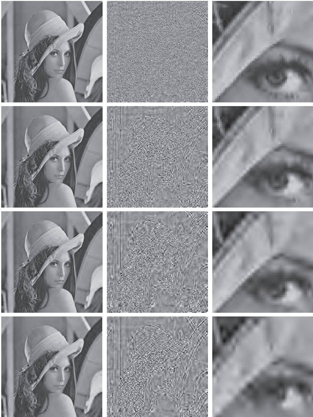
FIGURE 8.46 Four JPEG-2000 approximations of Fig. 8.9(a). Each row contains a result after compression and reconstruction, the scaled difference between the result and the original image, and a zoomed portion of the reconstructed image. (Compare the results in rows 1 and 2 with the JPEG results in Fig. 8.29.).
