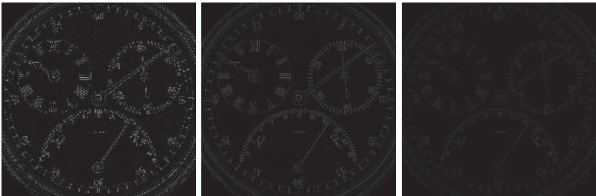
FIGURE 2.31 (a) Difference between the 930 dpi and 72 dpi images in Fig. 2.23. (b) Difference between the 930 dpi and 150 dpi images. (c) Difference between the 930 dpi and 300 dpi images.
