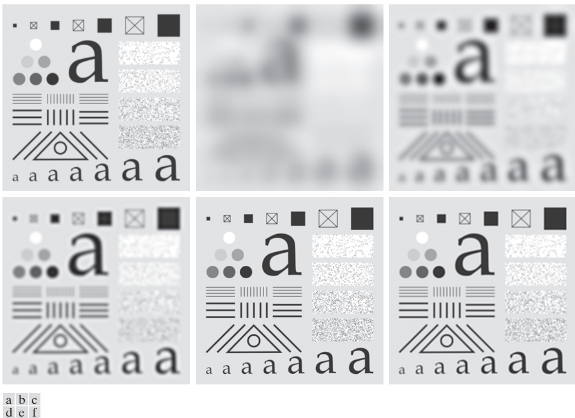
FIGURE 4.46 (a) Original image of size 688 \times 688 pixels. (b)–(f) Results of filtering using BLPFs with cutoff frequencies at the radii shown in Fig. 4.40 and n = 2.25 . Compare with Figs. 4.41 and 4.44. We used mirror padding to avoid the black borders characteristic of zero padding.
