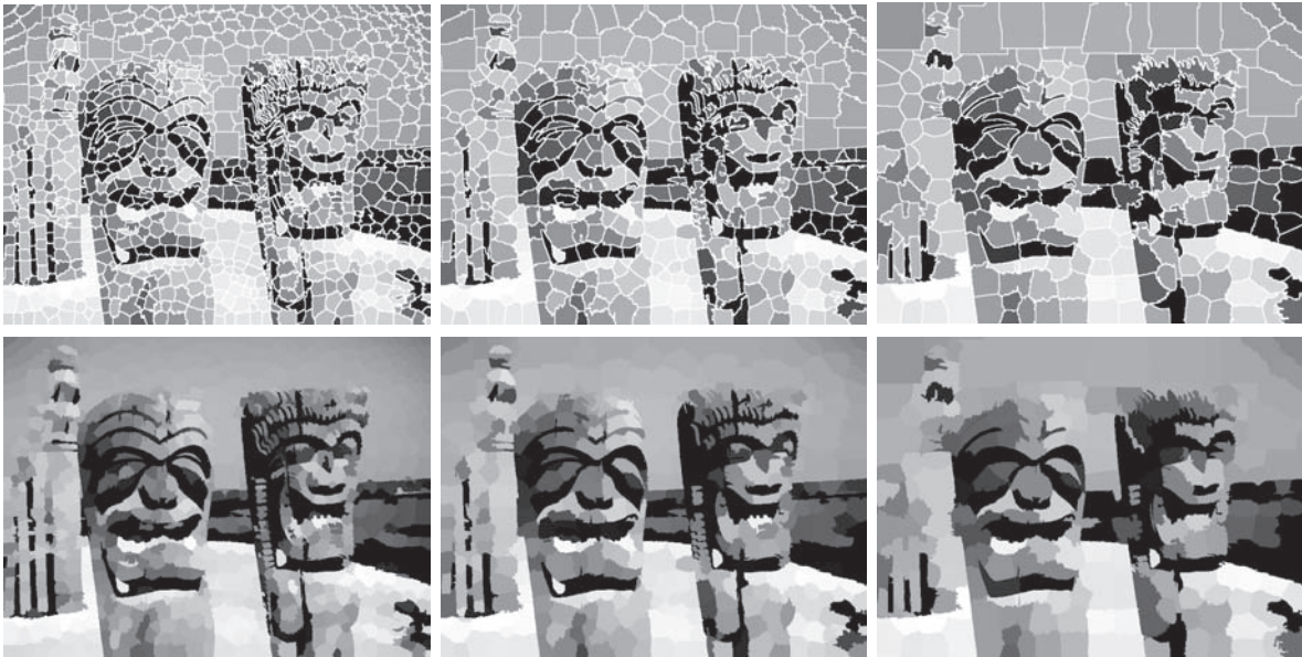
FIGURE 10.51 Top row: Results of using 1,000, 500, and 250 superpixels in the representation of Fig. 10.50(a). As before, the boundaries between superpixels are superimposed on the images for reference. Bottom row: Superpixel images.
