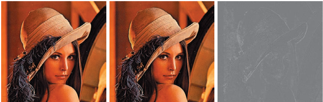
FIGURE 6.39 Image sharpening using the Laplacian. (a) Result of processing each RGB channel. (b) Result of processing the HSI intensity component and converting to RGB. (c) Difference between the two results.
