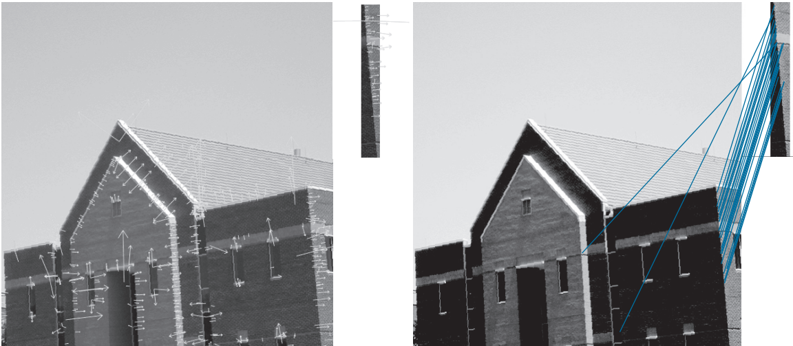
FIGURE 11.64 (a) Keypoints for the rotated (by 5^\circ ) building image and for a section of the right corner of the building. The subimage is a separate image and was processed as such. (b) Corresponding keypoints between the corner and the building. Of the 26 matches found, only two are in error.
