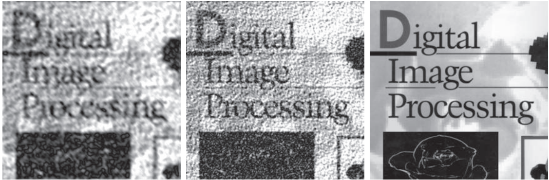
FIGURE 5.30 Results of constrained least squares filtering. Compare (a), (b), and (c) with the Wiener filtering results in Figs. 5.29(c), (f), and (i), respectively.
