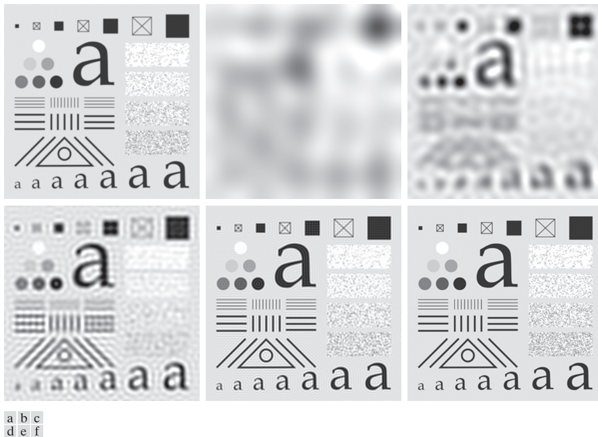
FIGURE 4.41 (a) Original image of size 688 \times 688 pixels. (b)–(f) Results of filtering using ILPFs with cutoff frequencies set at radii values 10, 30, 60, 160, and 460, as shown in Fig. 4.40(b). The power removed by these filters was 13.1, 7.2, 4.9, 2.4, and 0.6% of the total, respectively. We used mirror padding to avoid the black borders characteristic of zero padding, as illustrated in Fig. 4.31(c).
