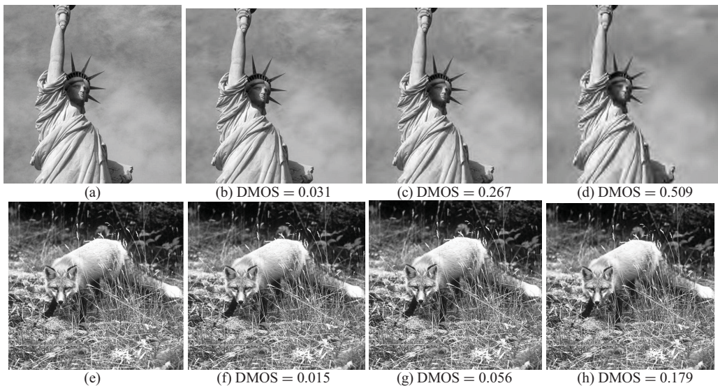
Fig. 2. Effect of distortion on image with relatively more smooth areas and more textured areas (these images are from CSIQ image database). First row: (a) original image “lady_liberty,” (b) JPEG 2000 distorted image for the first distortion level, (c) JPEG 2000 distorted image for the second distortion level, and (d) JPEG 2000 distorted image for the third distortion level. Second row: (e) original image “foxy,” (f) JPEG 2000 distorted image for the first distortion level, (g) JPEG 2000 distorted image for the second distortion level, and (h) JPEG 2000 distorted image for the third distortion level. The respective subjective scores in the form of difference mean opinion scores (DMOS) have been indicated below each distorted image.
